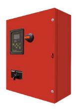
**Description**—Firetrol® FTA550E XG Jockey Pump Controllers are intended for use with fire pump systems. They are used for pressure maintenance in fire pump installations to prevent unnecessary operation of the main fire pump.
